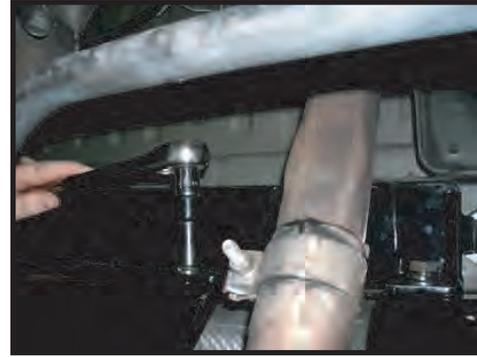
6. Tighten the body mount nuts and bolts loosened in Step 1. Push up on Skid Plate until the horizontal tabs are contacting the rear crossmember, and tighten the bumper mounting bolts.
