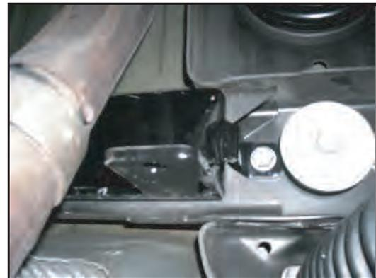
3. 2010-2011 vehicles will need to use supplied M10 bolt, Washer and Nut Plate to install mounting bracket. Slide nut plate on top of frame cross member. Place M10 spacer between frame and mounting bracket. Insert M10 bolt and washer. Start bolt into nut plate but do not tighten.
