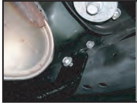
5. Install M12 Bolts and Washers through the Mounting Bracket and into the Skid Plate. Once all 3 have been started, tighten them.
